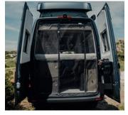
HYMER insulation and insect screen for the rear doors
